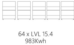
➤ **Max. 983kWh (64 modules) in parallel**
